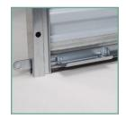
The slide bolt lock assembly affixed to the bottom bar at each end of the door curtain fastens through the guide to securely keep the door locked and in the down position. Padlocks can be attached to the slide to further secure the door.
